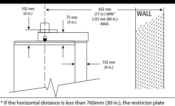
\* If the horizontal distance is less than 760mm (30 in.), the restrictor plate must be installed (refer to installation manual for further details).
